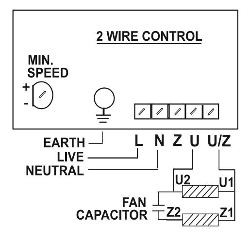
CONTROLLER WIRING DIAGRAM (for TK controllers Only) SINGLE PHASE SUPPLY
